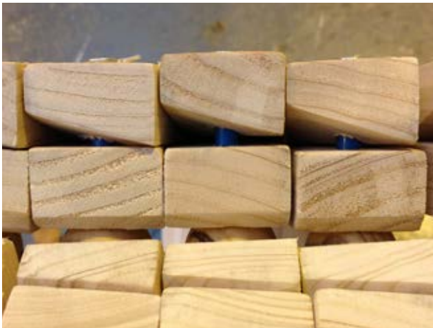
Chamfers in collapsed position
