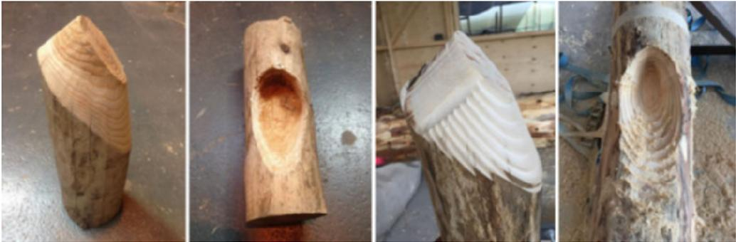
**Figure 9.** Development of the mortise and tenon connection.
