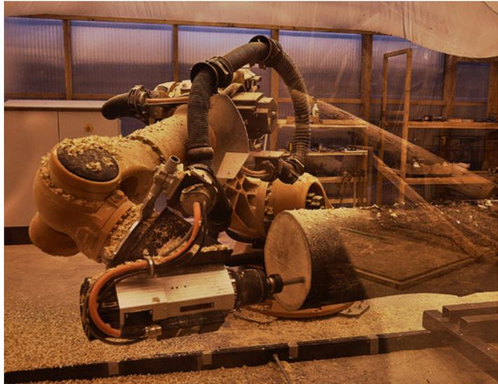
steps. Thirdly, a simpler set of planar 'seat' surfaces were defined and milled, to which smaller reinforcing timber truss members were screw connected.
